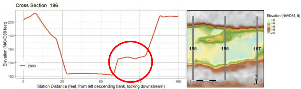
Figure 19. Cross-section 186, illustrating right floodplain berm development.
