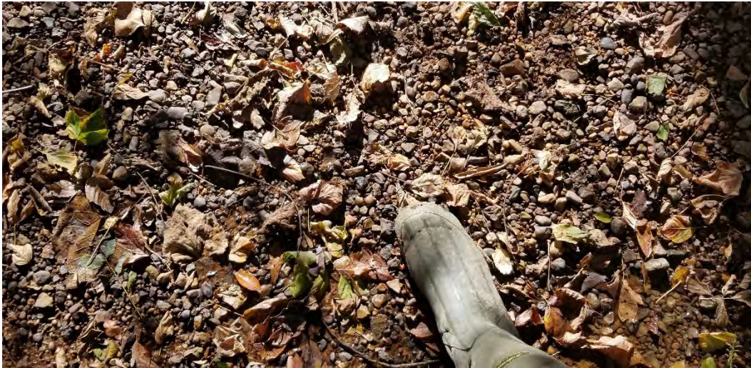
Figure 10. Johnson Creek upstream of State Route 301 culver with point bar material-small gravel to sand in Reach 3
